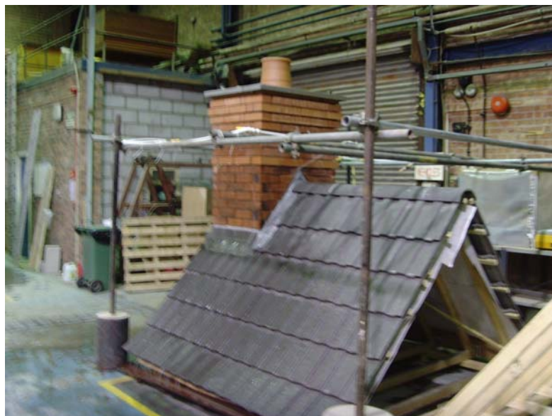
Plate 8 General View of Gable End Chimney under Water Tightness Testing
