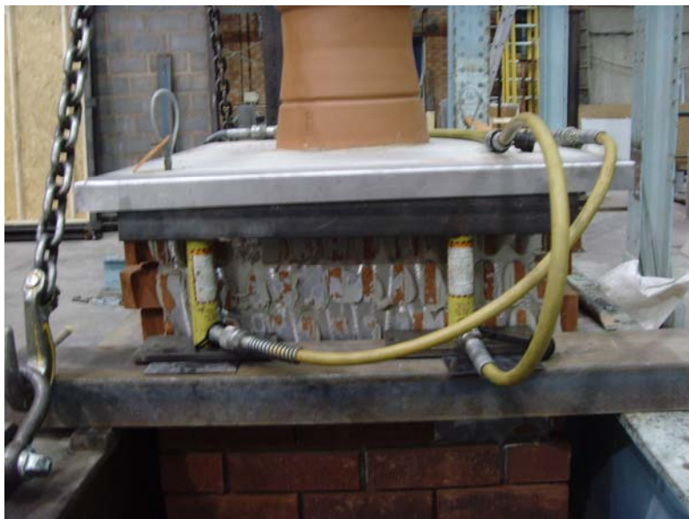
Plate 12 General View of Chimney Crown Pull-off Test
