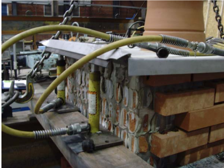
Plate 13 Failure of Crown by Bending of Overhang
