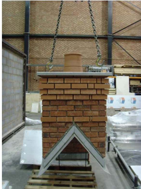
Plate 7 Chimney under Lifting Eye Test
